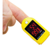
FIGURE 22.4 Portable pulse oximeter used to assess a person's arterial O 2 saturation. The finger probe shines a light through the fingertip, and the absorption of light due to the pulsing arterial blood is measured. The number on the left side of the display shows the percent saturation of hemoglobin in arterial blood (S O 2 ), and the number on the right side shows the HR.
