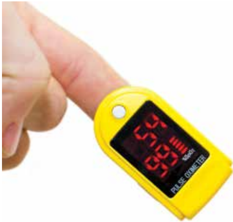
FIGURE 22.4 Portable pulse oximeter used to assess a person's arterial O_2 saturation. The finger probe shines a light through the fingertip, and the absorption of light due to the pulsing arterial blood is measured. The number on the bottom of the display shows the percent saturation of hemoglobin in arterial blood ( S_aO_2 ), and the number on the top shows the HR.
